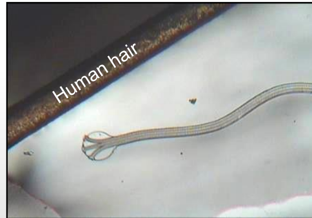
Intracortical electrode with 3 insulated Ti/W leads
